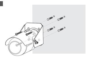
Installing using Wall Mount
